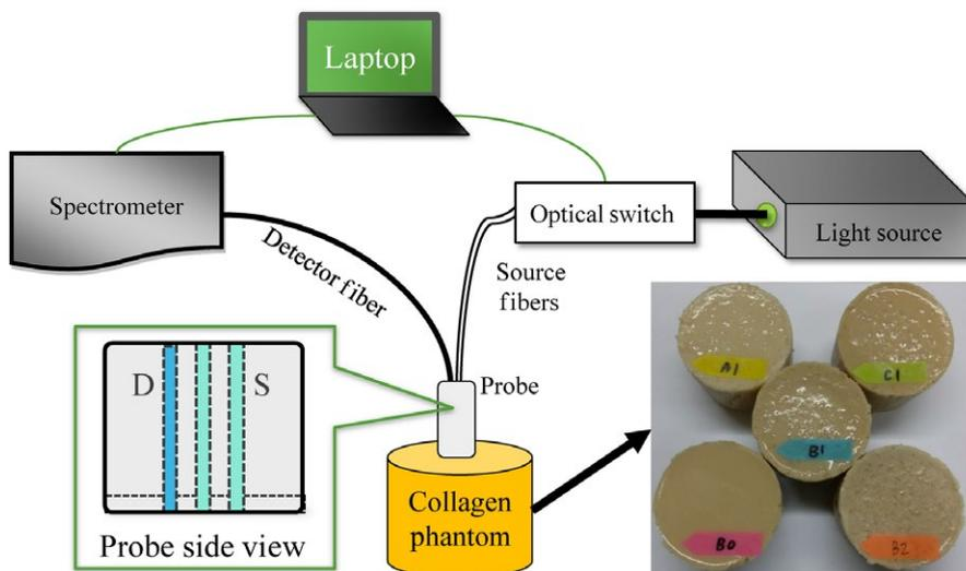
**FIGURE 1** The configuration of the DRS system and photo of collagen phantoms. D: detector fiber; S: source fibers [Colour figure can be viewed at [wileyonlinelibrary.com](http://wileyonlinelibrary.com)]
