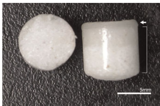
Figure 1. Biphasic cylindrical scaffold ready for cell seeding. About 1.5-mm depth of the top of the cylinder was the soft spongy chondral phase, and the remainder was the more rigid osseous phase. Left, top view; right, side view. (Arrow, chondral phase; bracket, osseous phase).
